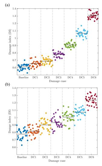
**Fig. 15.** Evolution of daily damage index (450 events/day) during progressive bridge condition change (every 30 days), for Scenario-2. Solid line indicates 30-day average value, using signals from: (a) tractor response (b) trailer response.
