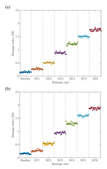
**Fig. 10.** Evolution of daily damage index (300 events/day) during progressive bridge condition change (every 20 days), for Scenario-1. Solid line indicates 20-day average value, using signals from: (a) tractor response (b) trailer response.
