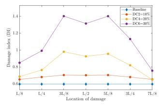
Fig. 16. Effect on damage index for different location of the bridge (Scenario-2).
