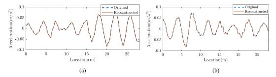
Fig. 5. Comparison of original and reconstructed vertical accelerations of two separate events for: (a) healthy and (b) damaged case.
