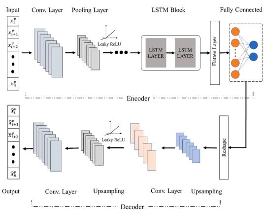
Fig. 2. Architecture of the proposed deep autoencoder model (DAE).
