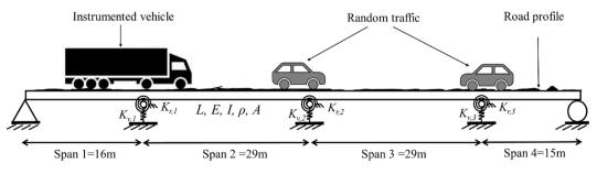
Fig. 17. Model of Voigt Drive I-5 bridge with instrumented vehicle and random traffic.
