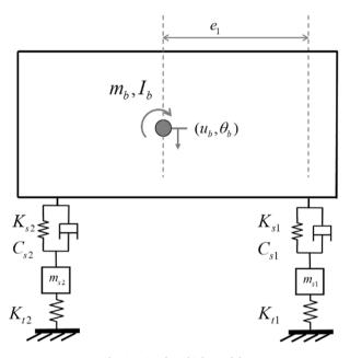
Fig. 19. 2-axle vehicle model.
