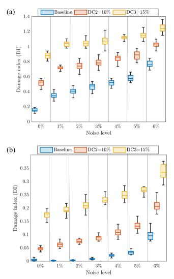
**Fig. 14.** Effect of measurement noise on the sensitivity of the damage index: (a) noise-free; (b) with noise.
