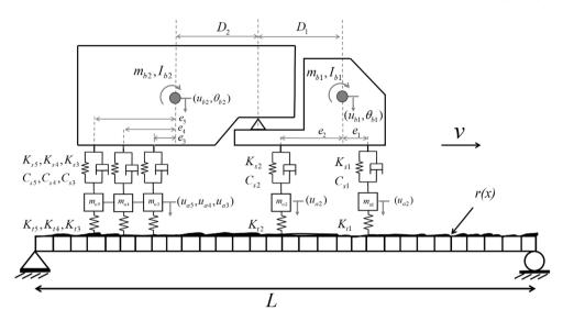
Fig. 3. Vehicle-bridge interaction model.
