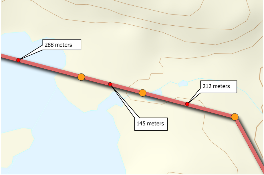
Figure 3.1: Line segment lengths. Main transmission line in red, towers as yellow points. Illustrative example using data from [111, 112].
