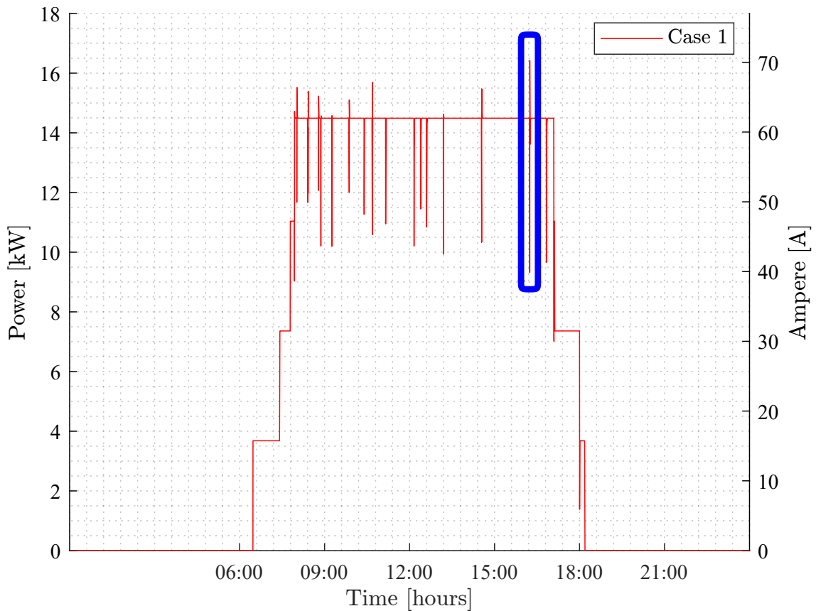
Figure A.1: Overview of P_{measured} , largest spike from case 1a marked in blue
