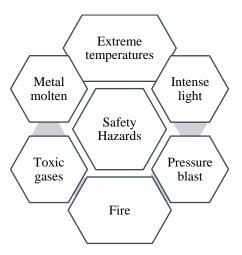
Figure 2-2: Arc flash safety hazard [7]
