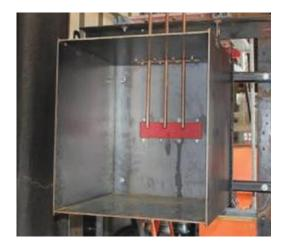
Figure 1-3: VCB - Vertical electrodes inside a metal enclosure [1]
