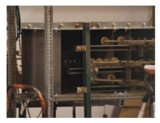
Figure 1-5: HCB - Horizontal electrodes inside a metal enclosure [1]
