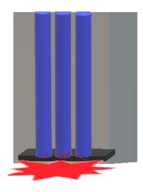
Figure 3-3: Vertical electrodes terminated in a metal enclosure's insulation barrier (VCCB) reproduced after [1, 11]
