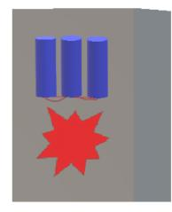
Figure 3-1: Vertical electrodes in a metal box enclosure (VCB) reproduced after [1, 11]
