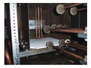
Figure 1-4: VCCB - Vertical electrodes terminated in an insulating 'barrier' inside a metal enclosure [1]
