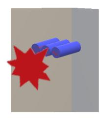
Figure 3-2: Horizontal electrodes in a metal enclosure (HCB) reproduced after [1, 11]
