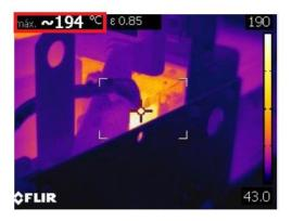
Figure 2-4: Circuit breaker terminal exceeding maximum allowable temperature, picture courtesy of BW Offshore
