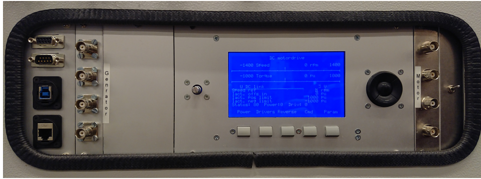
Figure 3.6: User interface for the DC-motor control unit (right) and the communication interface for the PicoZed processor card, as described in Chapter 3.4.2.
