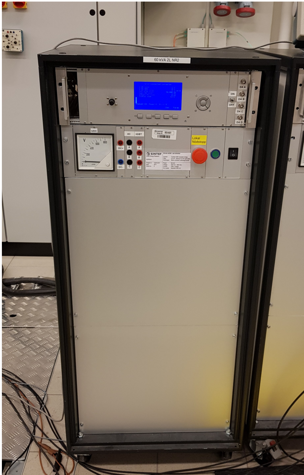
Figure D.2: Picture of the voltage source converter.
