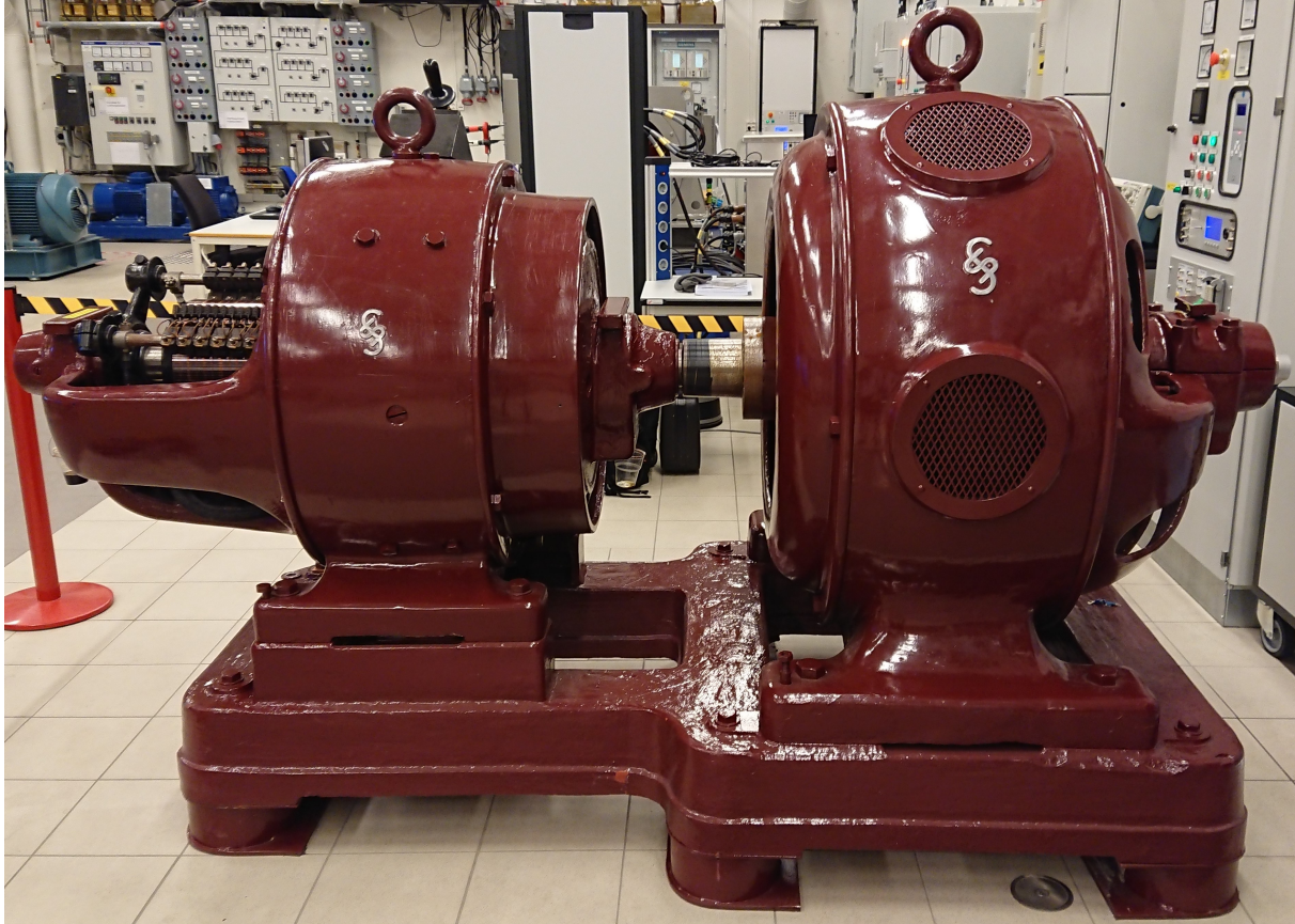
Figure 3.4: Picture of the Siemens-Schuckert motor/generator (45 kW / 75 kVA) set.
