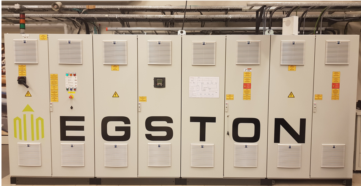
Figure D.3: Picture of the EGSTON 200 kVA power amplifier.
