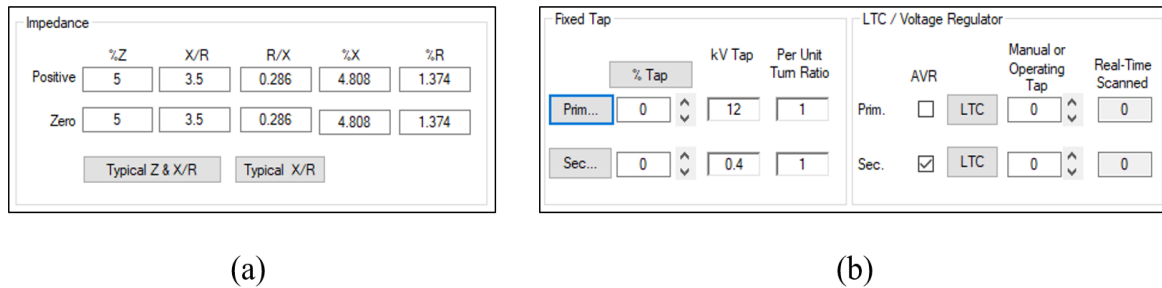
Figure 4-12 Tabs showing the (a) impedance and (b) transformer tap values according to requirements
