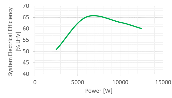
Figure 13: System efficiency with respect to Lower Heating Value (LHV) as a function of power output for a 10 kW SOFC system with some "overrun" capabilities. Kindly provided by Ceres Power.
