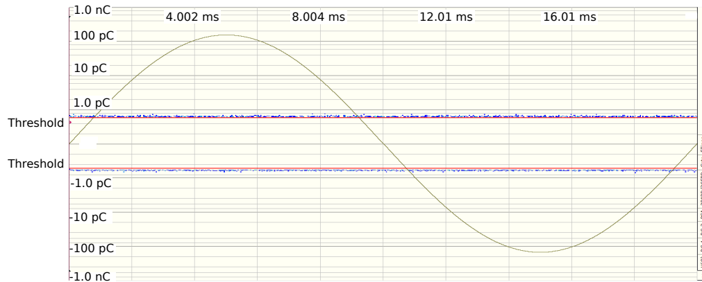
Figure 4.7: 10 kV DC test at 77 °C with C_s = 179 \text{ pF} and C_d = 5.75 \text{ nF} with the PET disk sample.
