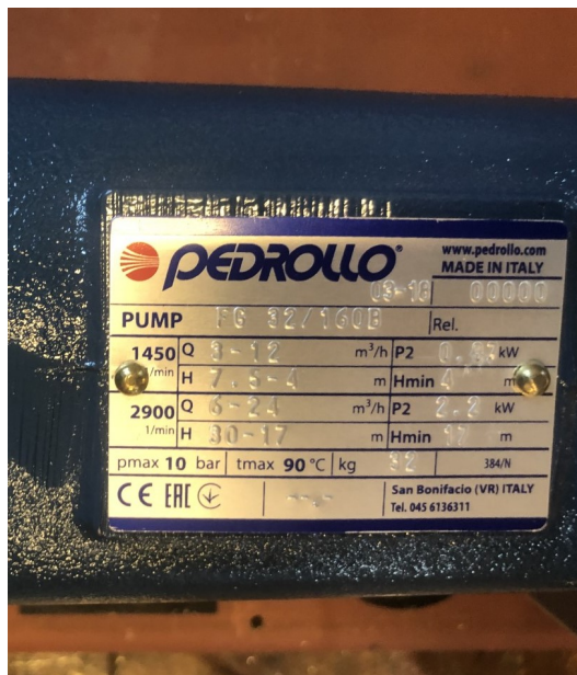
Figure 2: Nameplate data of the pump used as turbine
