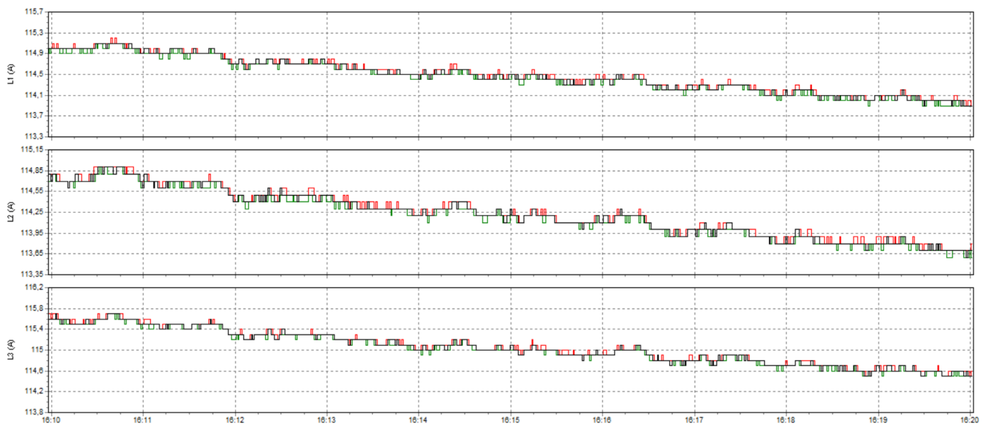
Figure C.1.3: The current [A] applied during the beta temperature measurement for nominal current.
