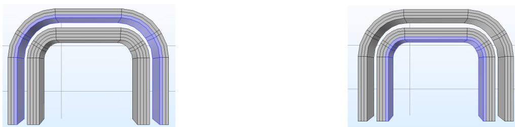
(a) The definition of the inner primary winding using Coil. (b) The definition of the inner secondary winding using Coil.
