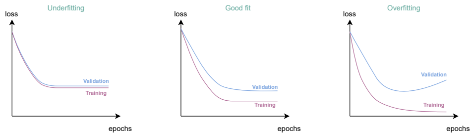
Figure 2.10: Underfitting, good fit and overfitting. A model is underfit if the training loss and validation loss are close to each other. It is a good fit if training loss is slightly lower than validation loss. A much lower training loss than validation loss indicates an overfit. Here epochs represents the training steps.
