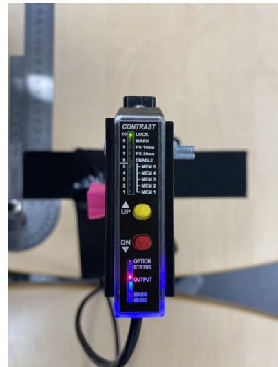
Figure 30: Contrast scale for the photoelectric sensor.
