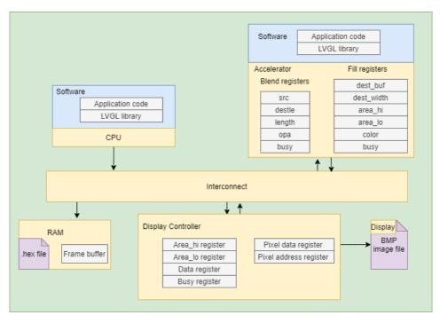
**Figure 5.2:** Graphics subsystem with display controller having DMA and hardware accelerator to offload some application code from the CPU
