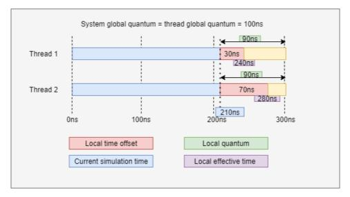
Figure 4.3: Illustration of temporal decoupling concept with time quantum
