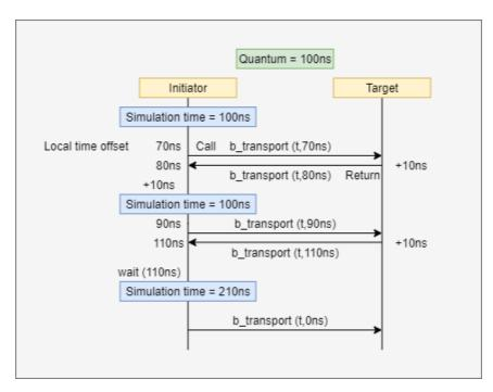
Figure 4.4: Blocking transport with temporal decoupling synchronized implicitly
