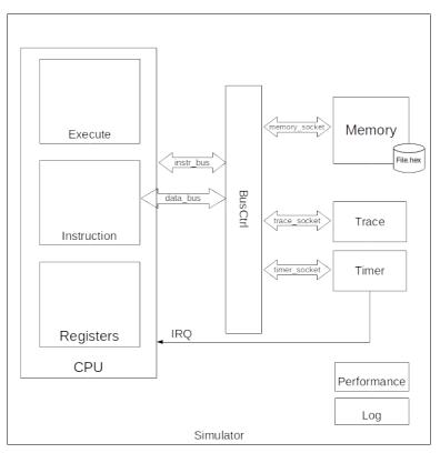
Figure 3.1: Structure of the base RISCV-ISA Simulator [18]
