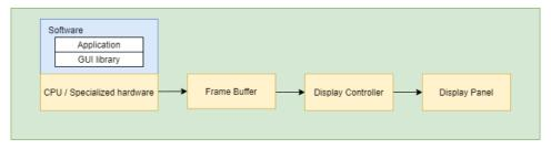
Figure 2.1: The data flow to rendering graphics in a graphics subsystem
