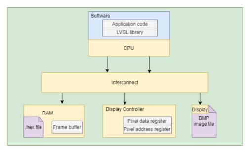
Figure 3.5: Graphics subsystem on the SystemC + TLM simulator
