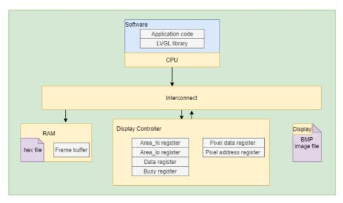
Figure 5.1: Graphics subsystem with display controller having DMA
