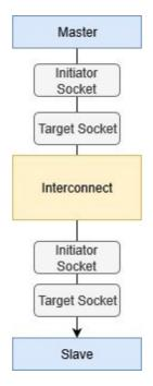
Figure 2.8: Representation of the flow of a TLM transaction from Initiator to Target
