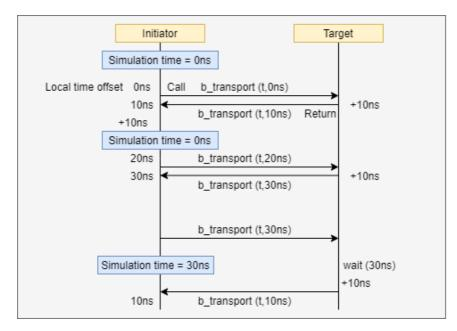
Figure 4.2: Blocking transport with temporal decoupling synchronized explicitly
