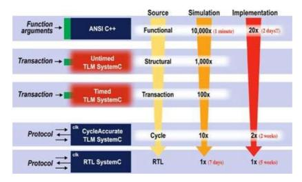
Figure 2.7: Implementation and simulation speeds at different levels of abstraction
