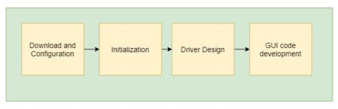
Figure 3.4: Steps to port LVGL for use in a project
