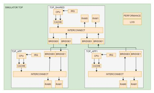
Figure 3.2: Structure of the Customized Simulator used in this thesis
