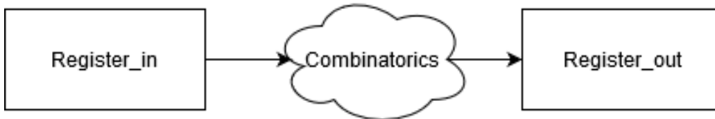
Figure 3.1: Illustrations of how combinatorial blocks are tested. A pattern is applied to the input register, and the output register is read. The values from the output register are compared to the expected value.
