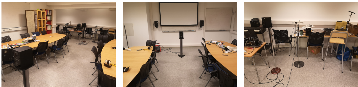
Figure 7.5.: Pictures of the measurement setup in the conference room showing microphone and loudspeaker placement.
