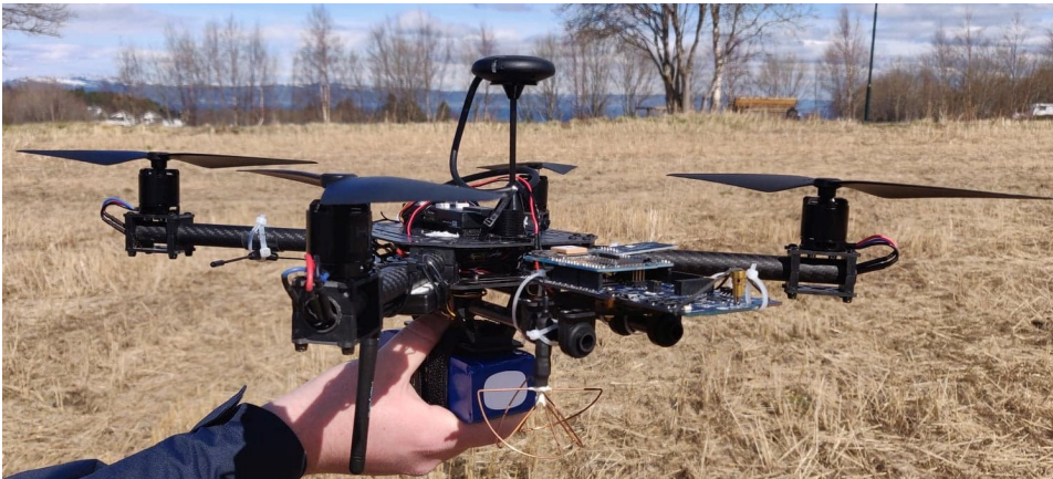
Figure B.3: Photograph showing the circularly polarized cloverleaf antenna connected to the central device and mounted on the quadcopter drone.
