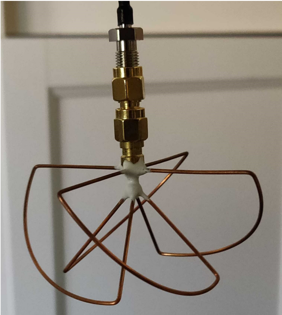
Figure B.2: Photograph showing the circularly polarized cloverleaf antenna used as the receiving antenna on the UAV.
