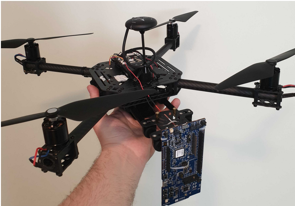
Figure B.1: Photograph of the quadcopter drone used in the experiments. The picture also show how the central device was equipped as the payload of the UAV.
