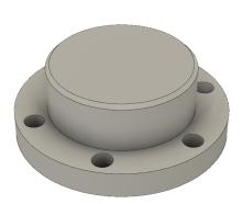
(a) 3D-model finished designed LED housing top, 6 bolts to hold top and bottom together with o-ring in between for water- mounting to inner lid and provide wiring to proofing
