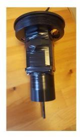
**Figure 8.4:** Protective cover over limit switch holder and linear actuator. Reinforced with tape to smooth sharp edges, mitigate risk of wires and connectors to get tangled
