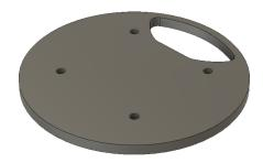
**Figure 6.5:** Show the removed section of inner lid to provide access for wiring to the PCB
