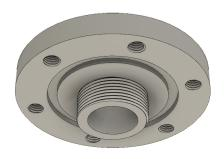
(b) 3D-model finished designed LED housing bottom, 6 bolts to hold top and bottom together with o-ring in between for waterproofing, o-ring between bottom and outer lid, and a threaded cylindrical tube for LED
