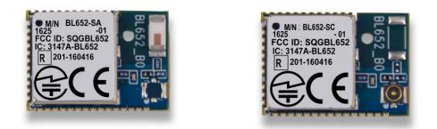
**Figure 3.2:** BL652 Radio module with two antenna configurations; **Left:** Ceramic chip monopole antenna, **Right:** MHF4 connector. Reproduced from datasheet [21]
