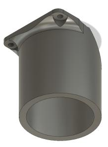
**Figure 6.4:** Protective Cylinder Cover to avoid wires from getting tangled in the lead screw of linear actuator and limit switch holders, mounted on two M4 bolts underneath the stepper motor block
