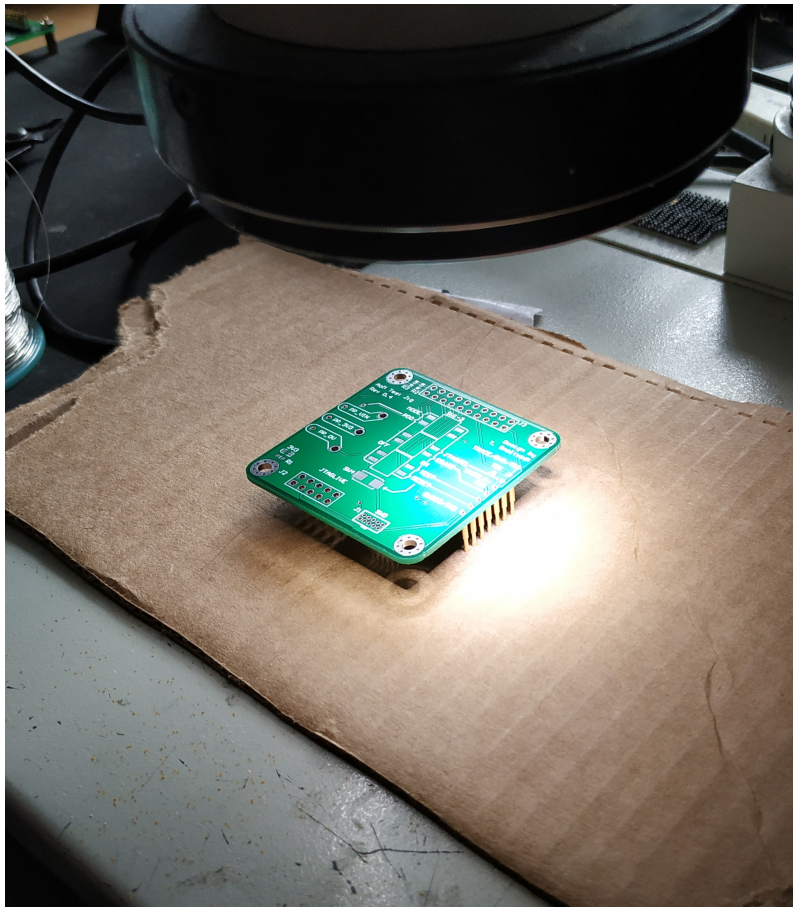
Figure 4.1: Assembly of test jig. Cardboard was used to hold pogo pins in place during soldering.
