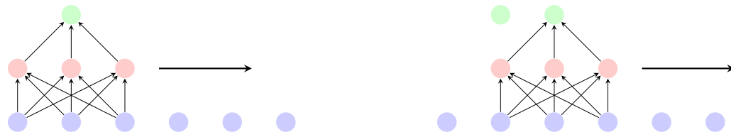
Figure 3.6: An illustration of how a one-dimensional convolutional layer works. The blue circles represent the input to the convolutional layer, the red circles represent units that make up the convolutional layer, the green circles represent the output of the convolutional layer, the thin arrows between units represent the weighted sum, and the thick arrow represents the sliding of the filter over the input.
