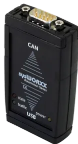
The CAN USB converter used for this test was systec CAN (IEC 61131-3)
