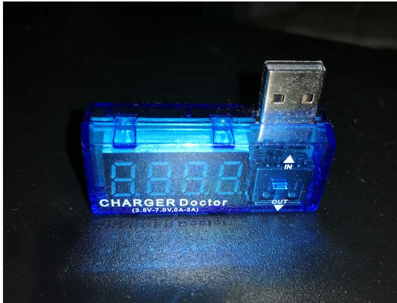
Figure 4.1.: Adafrit Charger Doctor, an Inline Multimeter
