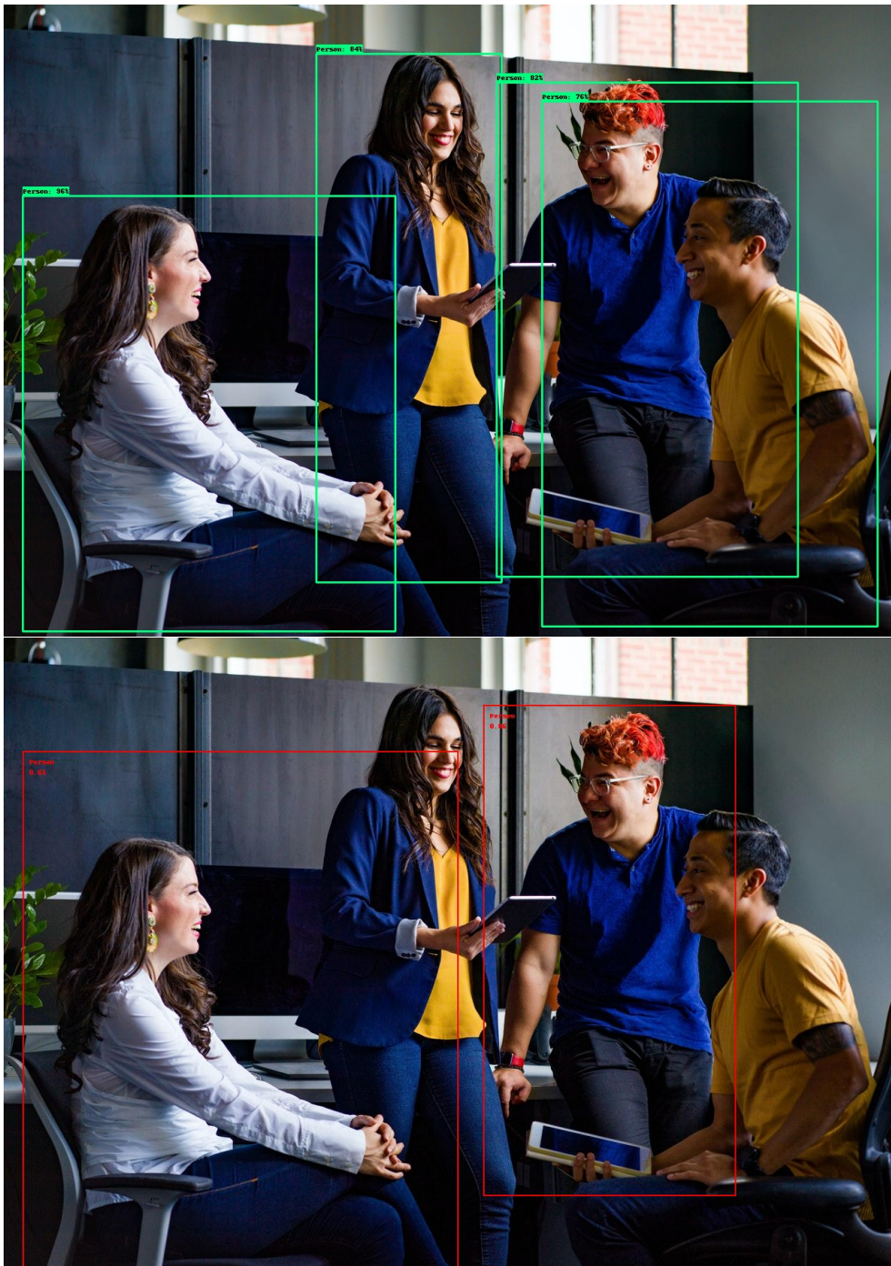
Figure 5.6: Detection result using the Non-Quantized Mobilenet model. Top: using the frozen graph exported from Object Detection API. Bottom: using the exported TFLite formatted model. Both tested with a threshold set to 0.4, Image is "Group of People Sitting Inside Room" by JopWell, Licensed as "Free to Use"
