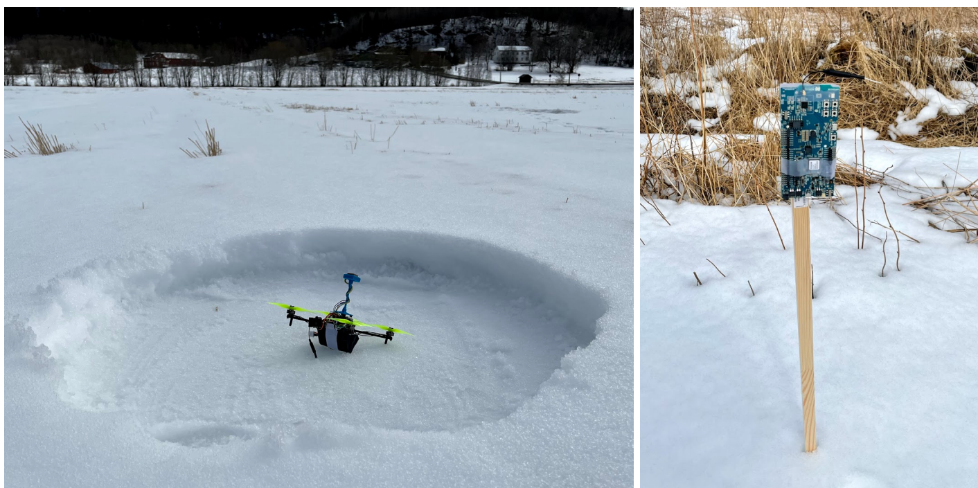
(a) Drone and attached nRF with antenna hanging down.
