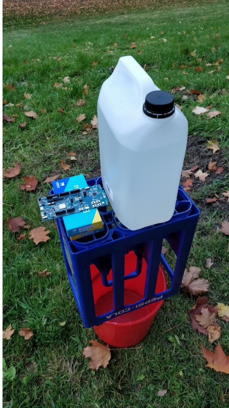
Figure 5.5: nRF52833 range test 2 water container setup.
