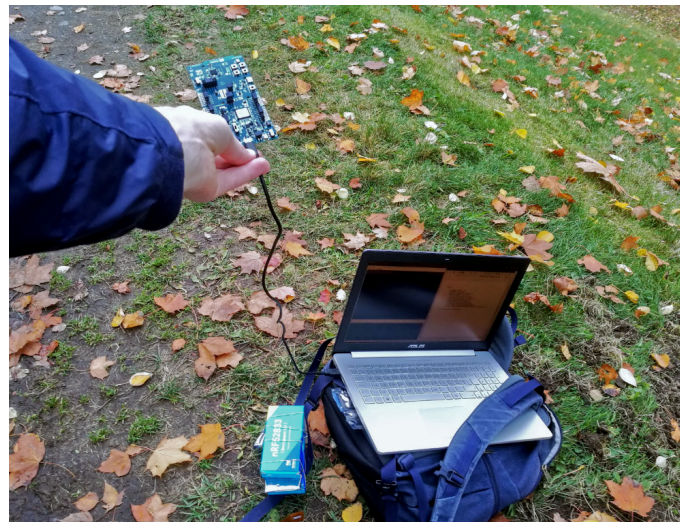
Figure 5.2: Position of the nRF52833 development kit simulating the drone.
