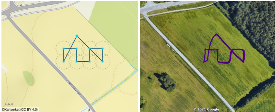
(a) Route planned in Radio Sheep GCS. (b) Actual flight performed by the drone.
