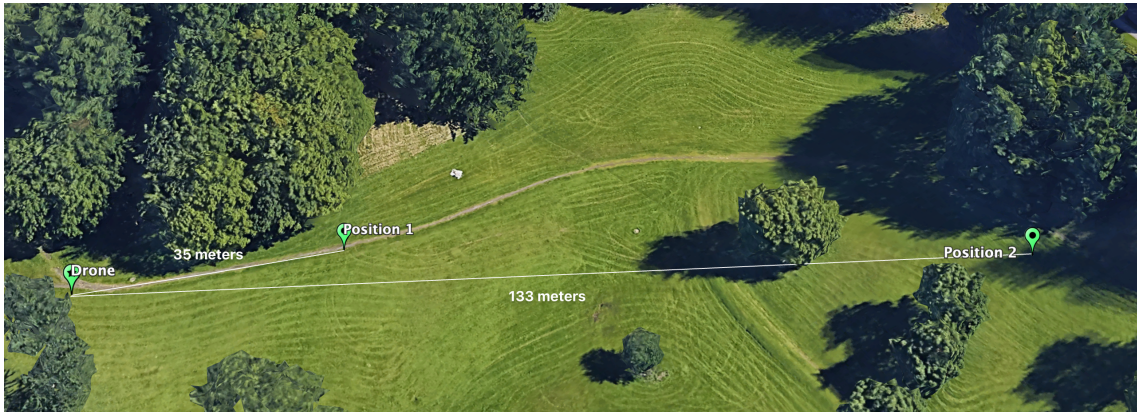
Figure 5.4: nRF52833 range test 2 locations.
