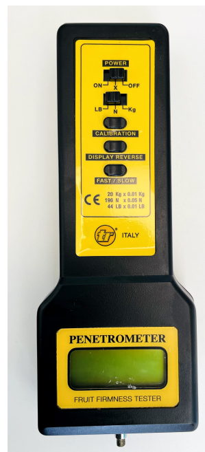
Figure 5.6: Penetrometer used for the firmness measurements.
