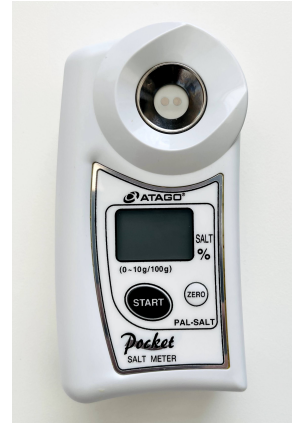
Figure 5.9: Pal-Salt: Digital hand-held salt meter by Atago.
