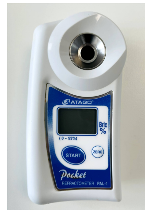
Figure 5.8: Digital Atago Pal-1 Digital pocket refractometer.
