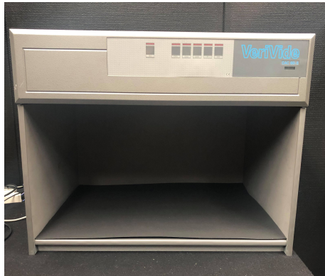
(a) Veri Vide CAC 60-5 light booth for simulating lighting conditions
