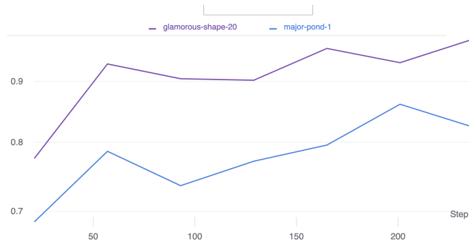
Figure 5.6: Average F1 score of all the fields. The first Yolov3 model vs the latest. Glamorous-shape-20 is name of the latest model.
