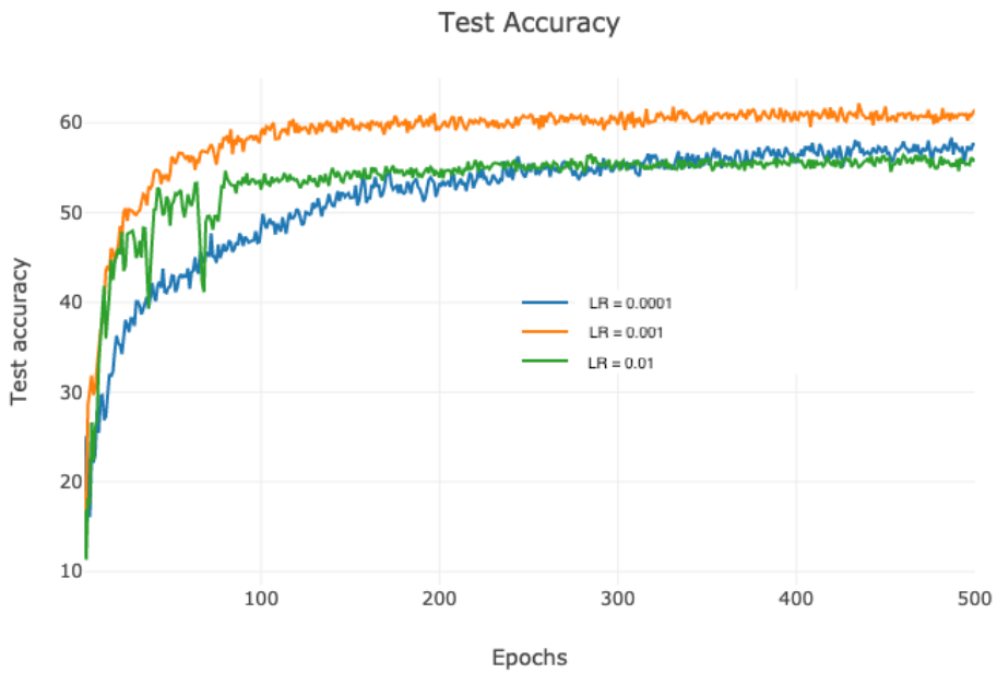
Figure 6.4: Test accuracy for CapsNet model trained for 500 epochs with one sample per class on the MNIST dataset and a batch-size of 1. The different lines are the Capsnet model trained with different learning rates from 0.01 to 0.0001.
