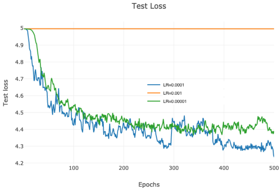
Figure 6.2: Test loss for CNN model trained for 500 epochs on MNIST with one sample per class on the MNIST dataset and a batch-size of 1. The different lines are the CNN model trained with different learning rates from 0.001 to 0.00001.
