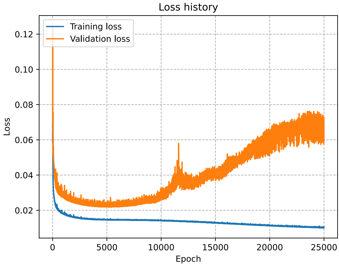
Figure 32: Training/validation loss during training using a single layered LSTM with 160 hidden units, 0.2 dropout rate and MAE loss over 25000 epochs. The first 10 epochs were removed from the graph because of high values compared to later values. Including these would make it harder to analyze the later values.
