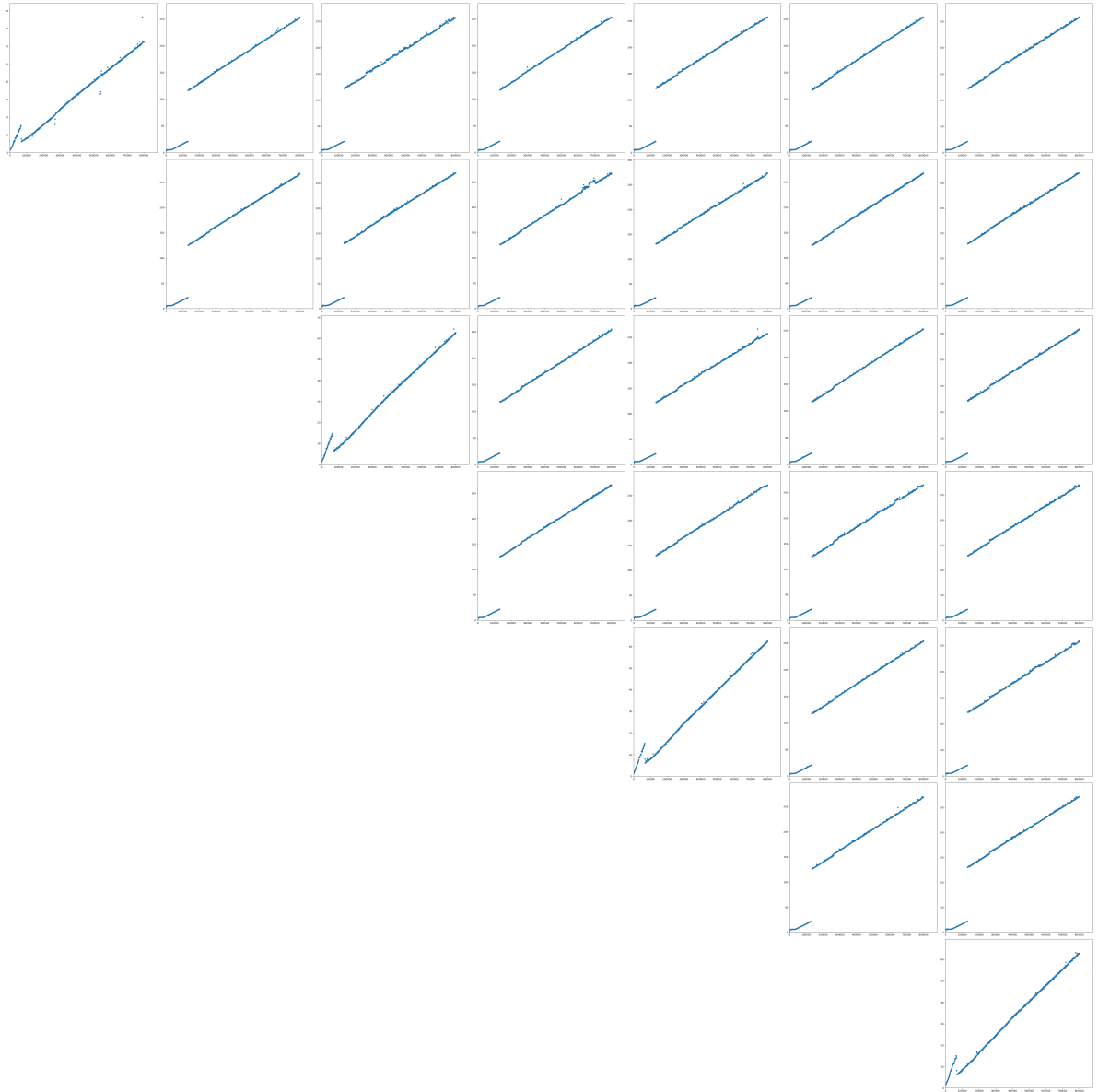
Figure 8.8: Communication matrix for 4 nodes on idun, with two ranks on each. We find the communication times are similar for all internode and intra node communication
