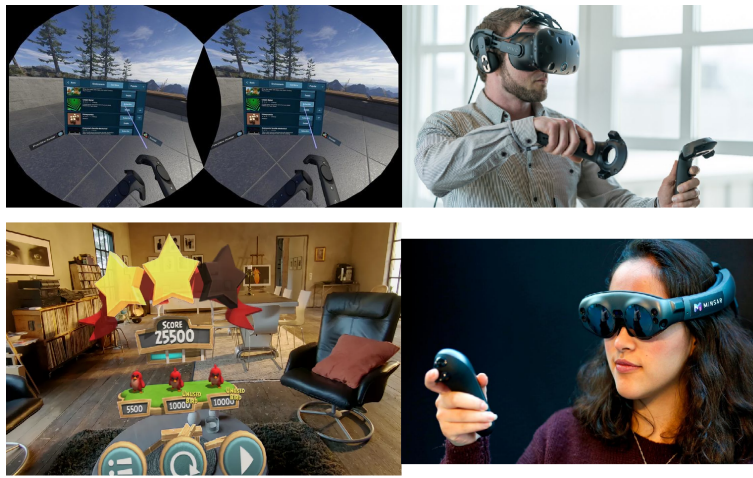
Figure 5: Top: Vive, bottom: magic leap. The Vive has a monitor for each eye, effectively separating the user from reality. The Magic leap uses the see-through display to superimpose the virtuality on top of reality, anchoring it in reality.
