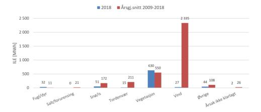
Figure 2.19: Overview of ILE on the transmission- and regional net caused by surroundings [Statnett, 2019b].
