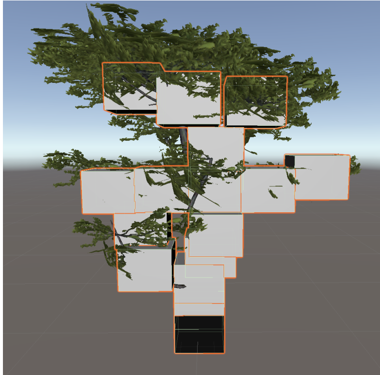
FIGURE 7.8: The trees are made up of a chain of nodes (cube meshes). Each node has specified the links to the next nodes that should burn. The HP and fuel values for the trunk of the tree is higher than the leaves and branches. The mesh renderer for each node is hidden, so the player does not see them in-game.
