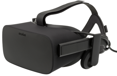
FIGURE 3.2: The Oculus Rift CV1 (Consumer Version 1), a virtual reality headset made by Oculus VR and released in 2016. Source: [28]
