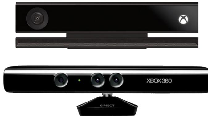
Figure 2.1: The Xbox One Kinect (top) and the older Xbox 360 Kinect (below) © Microsoft
