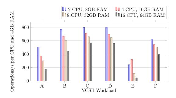
Figure 4.15: YCSB performance per CPU and 4GB RAM for three-node YugabyteDB clusters with serializable isolation on different instance sizes.
