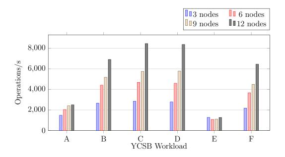
Figure 4.16: YCSB performance for YugabyteDB clusters with serializable isolation using different numbers of 4 CPU 16GB RAM nodes.
