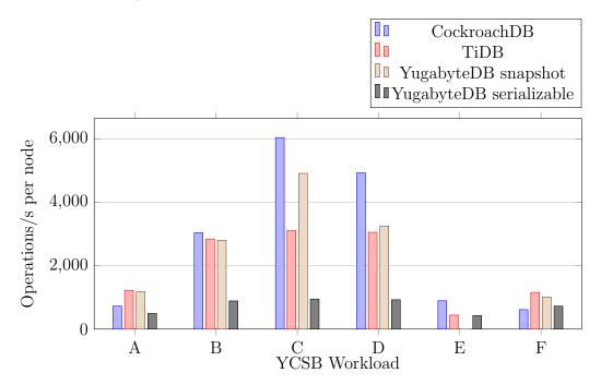
Figure 4.18: YCSB performance per node for minimal CockroachDB, TiDB and YugabyteDB clusters using 4 CPU 16GB RAM nodes.
