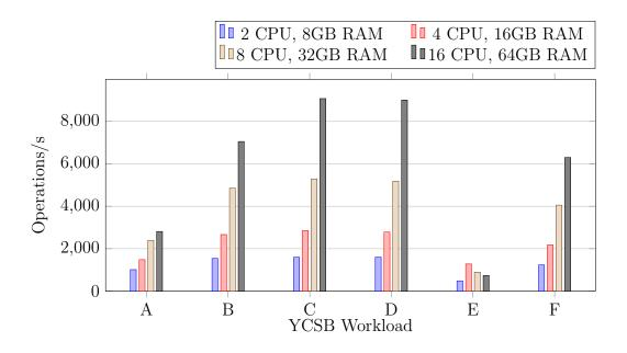
Figure 4.14: YCSB performance for three-node YugabyteDB clusters with serializable isolation on different instance sizes.
