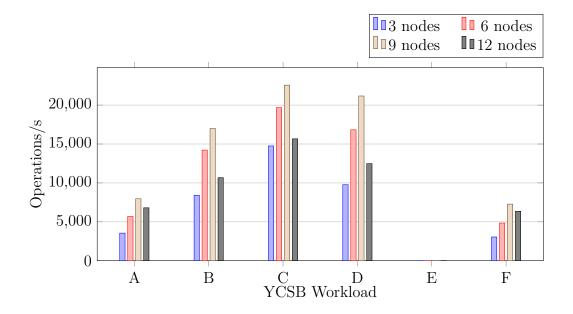
Figure 4.12: YCSB performance for YugabyteDB clusters with snapshot isolation using different numbers of 4 CPU 16GB RAM nodes.
