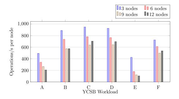
Figure 4.17: YCSB performance per node for YugabyteDB clusters with serializable isolation using different numbers of 4 CPU 16GB RAM nodes.
