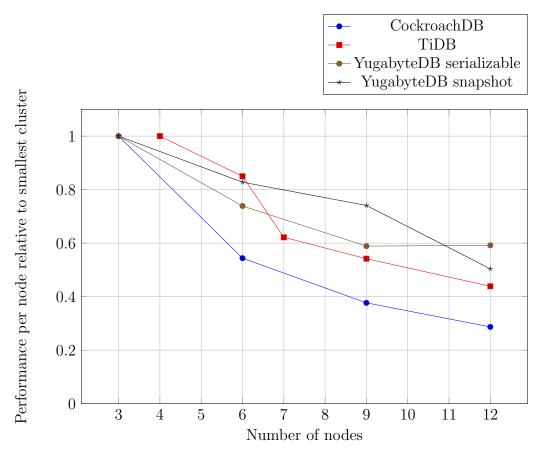
Figure 4.21: Comparison of performance per node for CockroachDB, TiDB and YugabyteDB when scaling horizontally. Performances are normalized to illustrate the cost of scaling by defining that minimal cluster of each database has a performance per node of 1.
