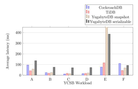
Figure 4.19: YCSB latencies for minimal CockroachDB, TiDB and YugabyteDB clusters using 4 CPU 16GB RAM nodes. The y-axis is cropped because YugabyteDB with snapshot isolation on workload E has a latency of over 30 seconds.
