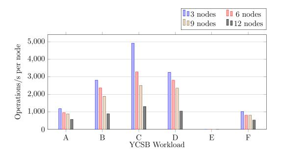
Figure 4.13: YCSB performance per node for YugabyteDB clusters with snapshot isolation using different numbers of 4 CPU 16GB RAM nodes.
