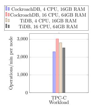
Figure 4.20: TPC-C performance per node for minimal CockroachDB and TiDB clusters using both 4 CPU 16GB RAM and 16 CPU 64GB RAM nodes. YugabyteDB is excluded because it was not able to run the TPC-C workload.
