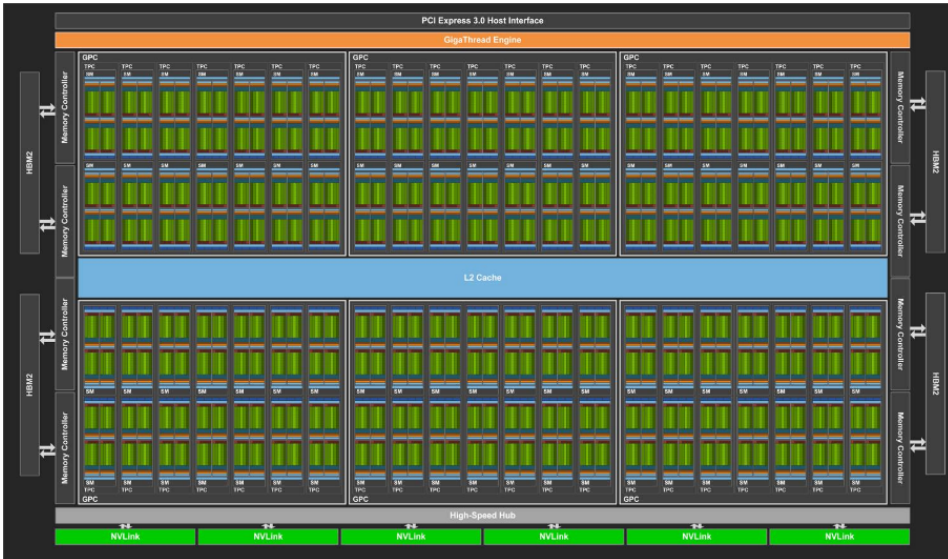
Figure 2.1: Overview of the NVIDIA Volta V100 GPU [1]. Note that this shows a full GV100 GPU with 84 streaming multiprocessors, and that the V100 mentioned and used in this work has 80 streaming multiprocessors available. With permission from NVIDIA.
