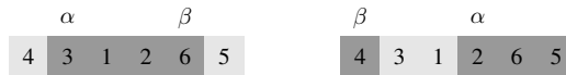
Figure 5.7: Two different examples on how the \alpha and \beta will determine which customers that will be inherited from parent 1.
