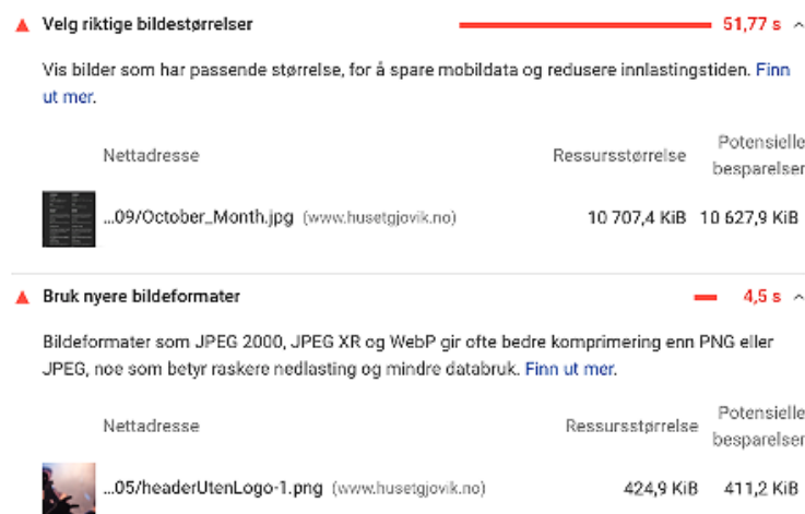
Figure 4.15: Screenshot from PageSpeed Insight showing detailed data for the images loaded on the mobile version. It shows that one image takes over 51 seconds to load, due to it being over 10 000 KiB in size.
