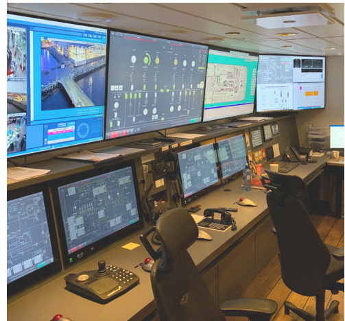
Figure 2.9 The engine control room aboard MS Newbuilt Explorer . Similar to the control room onboard MS Sister , but with more touch screens.
