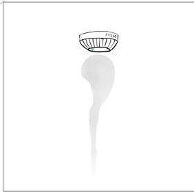
Smoke triggers a fire detector
