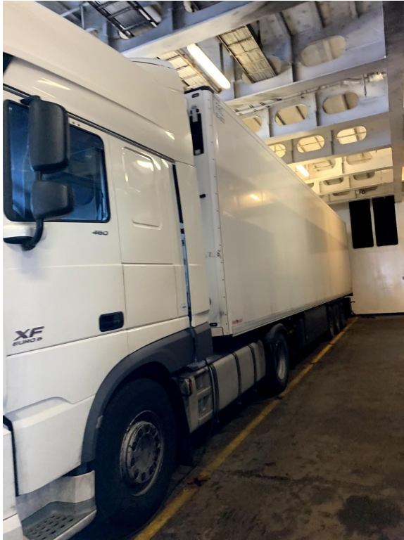
Images of a connected reefer. A reefer is a refrigerated or heated container. The pictured container is an electric reefer, a common source of fire aboard ro-ro-ships.
