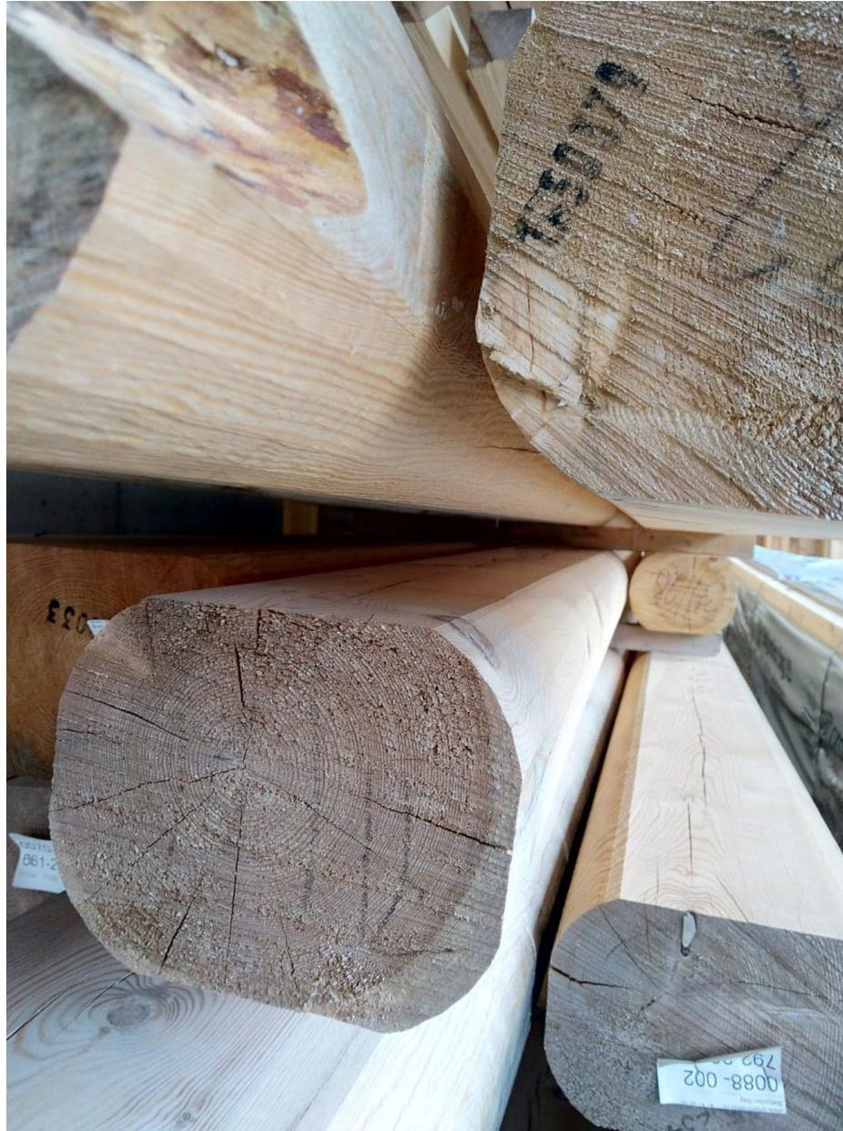
The two sawmills use heating systems to dry the water inside the wood. These systems are called kiln drying (M. Bøklepp, personal communication, February 13, 2020). They do this to hit the target of 16-20 percent moisture level. This translates to four weeks in the heating systems.
