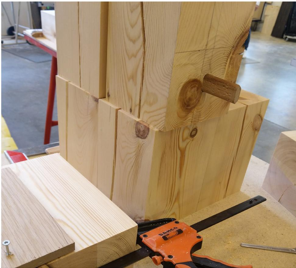
The wooden domino joints are a mass-produced element which differentiate allot from the natural looking pine. The domino joints look more like a technical element, while rest of the product expresses a more natural look. Based on these findings a second prototype was made. This prototype was the same size as the previous one, just with joints made from pine.
