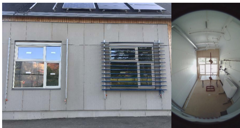
Figure 7-9 Facade of the test cell facility and a picture of the test chamber used.
