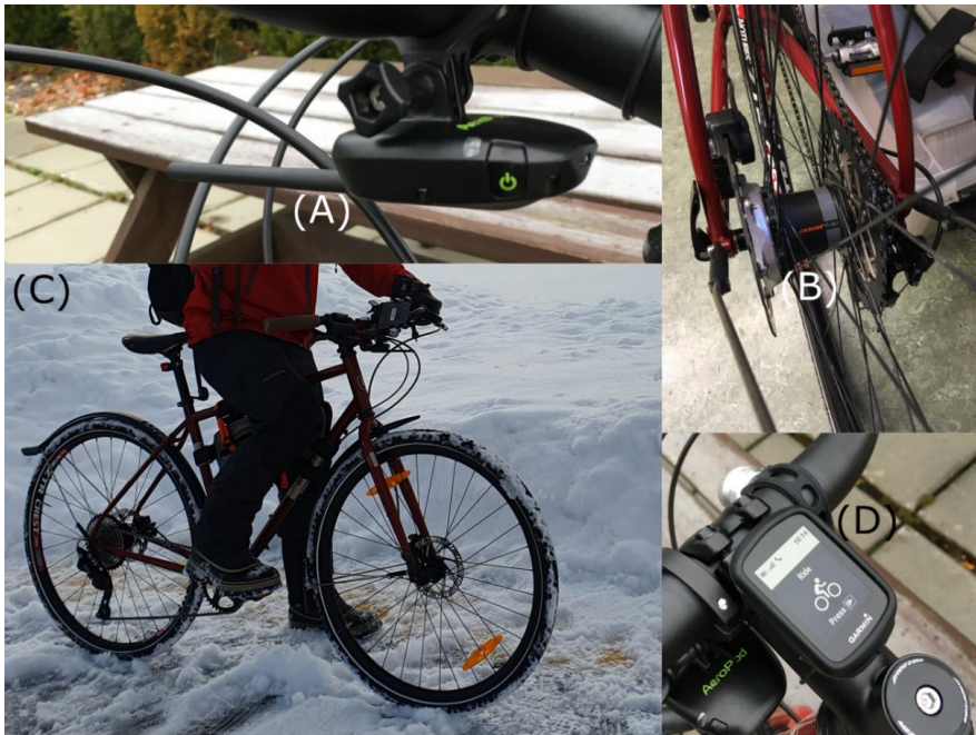
Figure 4: The instrumented bicycle (C), with air speed and slope sensor (A), pedaling power sensor (B), and GPS device (D).
