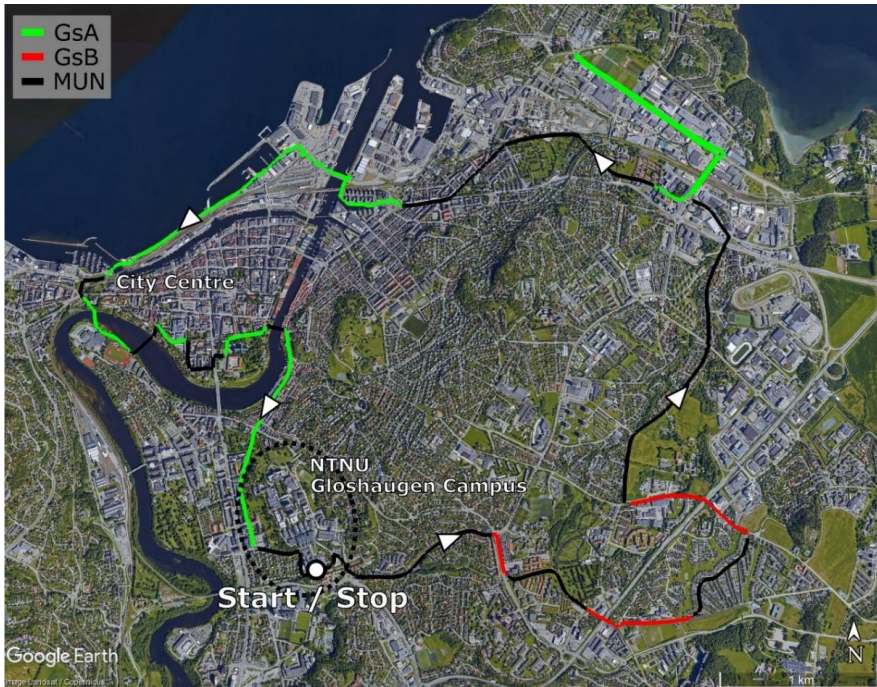
Figure 6: Satellite photo indicating the path and the winter maintenance standards for the rolling resistance test route.
