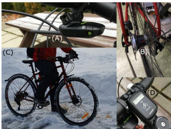
Figure 2: Airspeed, air density, and road slope sensor (A) Pedaling power sensor (B) Instrumented bicycle under winter conditions (C) GPS tracking device (D)
