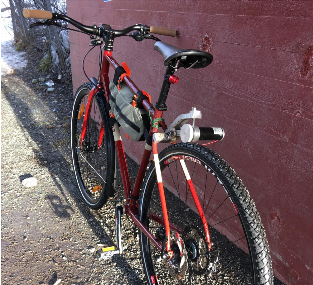
Fig. 4. Dynamo mounted to the bicycle for added rolling resistance.
