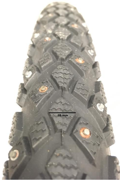
Figure 3: Tread of the tire used in the experiments (Schwable Marathon Winter Plus) Field measurements
