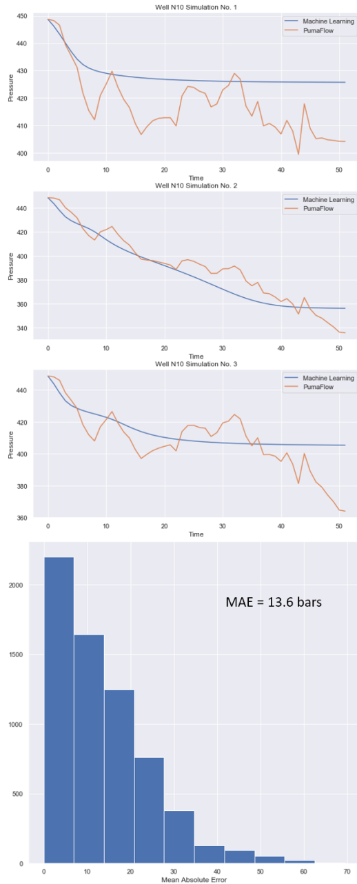
Figure 5.5: Experiment 1: This figure consists of plots to effectively understand ML-based simulation accuracy. The top three plots compare the ML-based simulation and PumaFlow TM physics-based simulations at sample wells and simulations from the training dataset. The bottom plot shows the error distribution while comparing the ML-based simulation to physics-based simulation at all wells and simulation from training dataset
