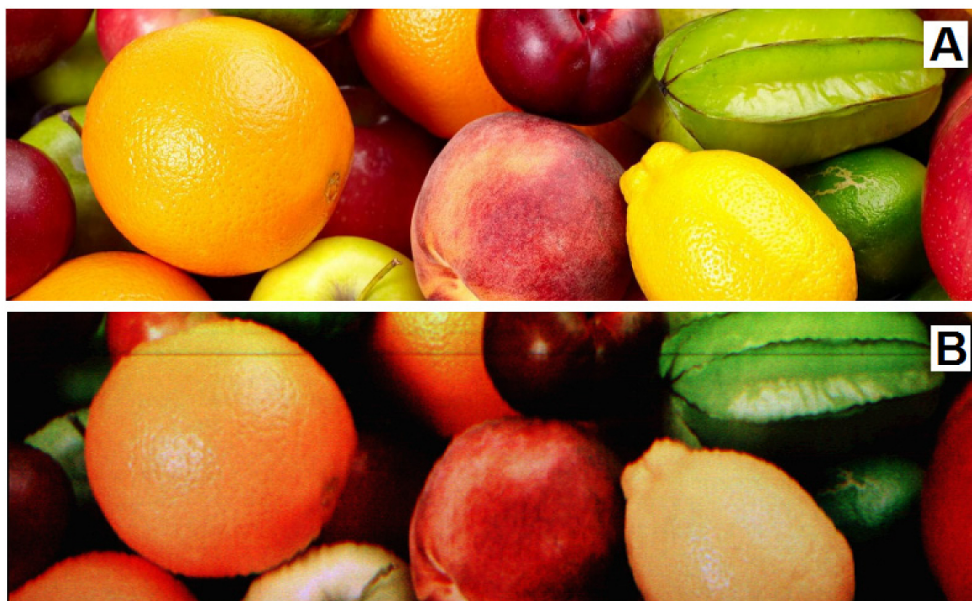
Figure 2.11: Handheld gimbal operation of the push-broom Hyperspectral Imager (HSI) - instrument (B). Panel (A): Target computer screen image. Panel (B): HSI RGB composite constructed by combining centre wavelength images at 490nm (blue), 552nm (green) and 620nm (red). Bandpass is 10nm for each colour channel.
