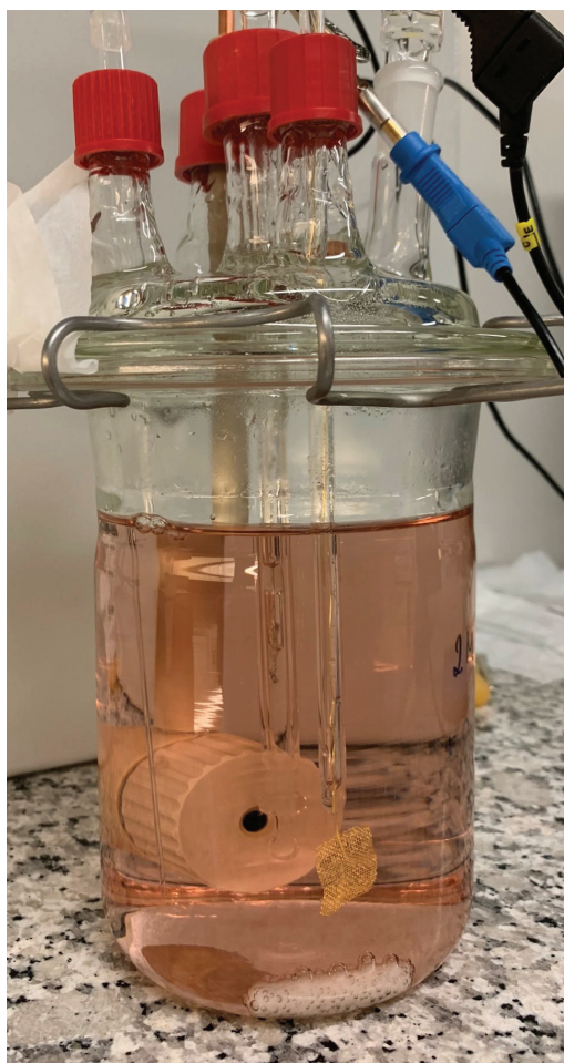
Figure 4.2: The cell used for conventional electrochemical measurements, containing a gold mesh CE, a reversible hydrogen reference electrode and a working electrode in a PEEK holder.
