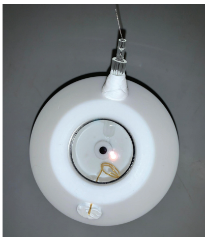
Figure 4.6: The electrochemical cell used for Raman spectroscopy as seen from above.
