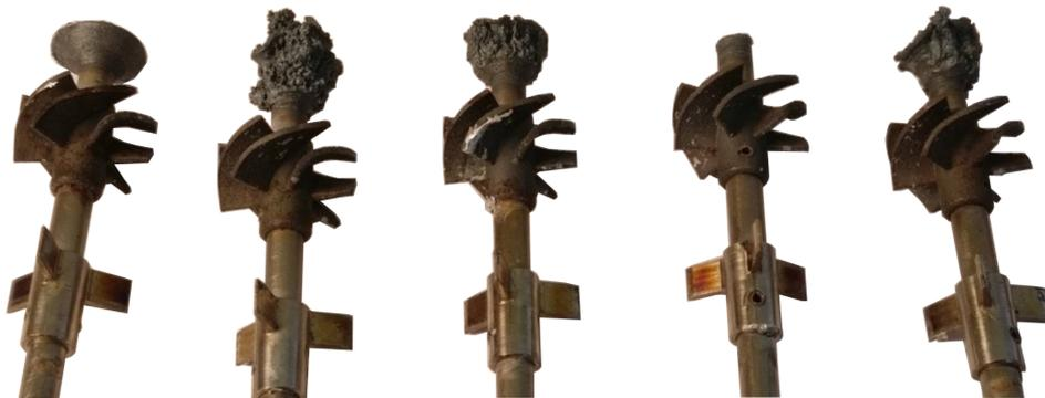
**Figure 1.5:** Damaged bluff bodies that were subject to instability induced flashback in a pressurized model annular combustor [Mazur et al. 2020].
