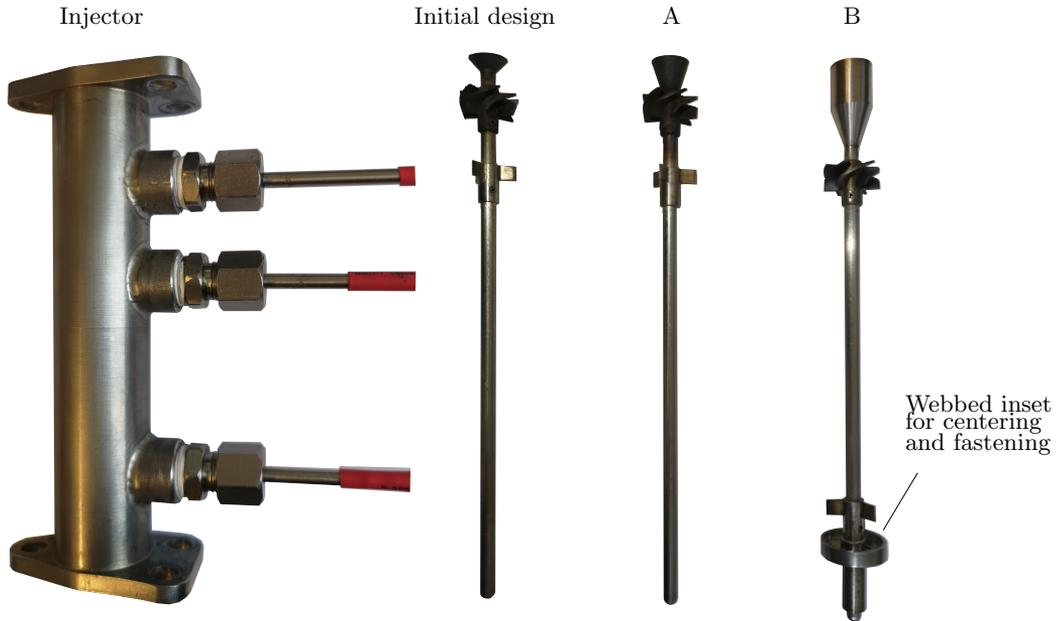
**Figure 3.6:** Left side: Injector pipe with microphones mounted. Right side: Evolution of the bluff bodies of the IPA combustor with the bluff bodies A and B which were used in this work.
