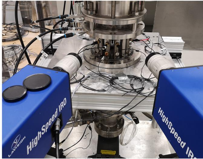
**Figure 3.15:** Camera arrangement of the IPA combustor.
