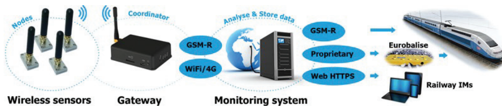
Fig. 1. Proposed condition monitoring system
