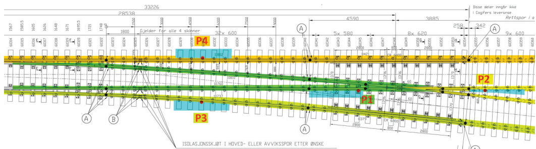
(b) Typical locations for a WS installation (P1, P3 and P4 may be in one line)
