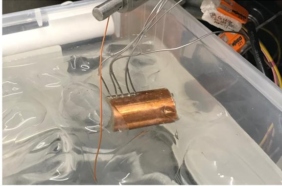
**Figure (3.8):** Ice bath calibration of the thermocouples embedded in the Cu cylinder, while the thermocouples are coupled to the circuit as they are during experiments.
