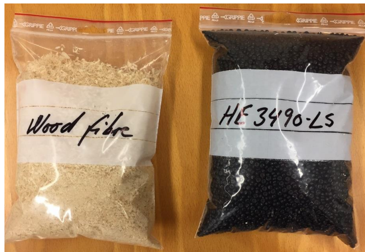
Figure 1. Raw materials employed for the production of WPC.
