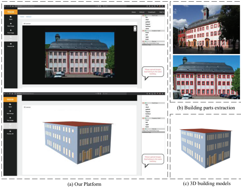
Figure 5. Results of our platform. (a) Interface of our platform. (b) Result of facade elements extraction, which is a middle part of our workflow. (c) Final result of 3D building modeling shown on our website.
