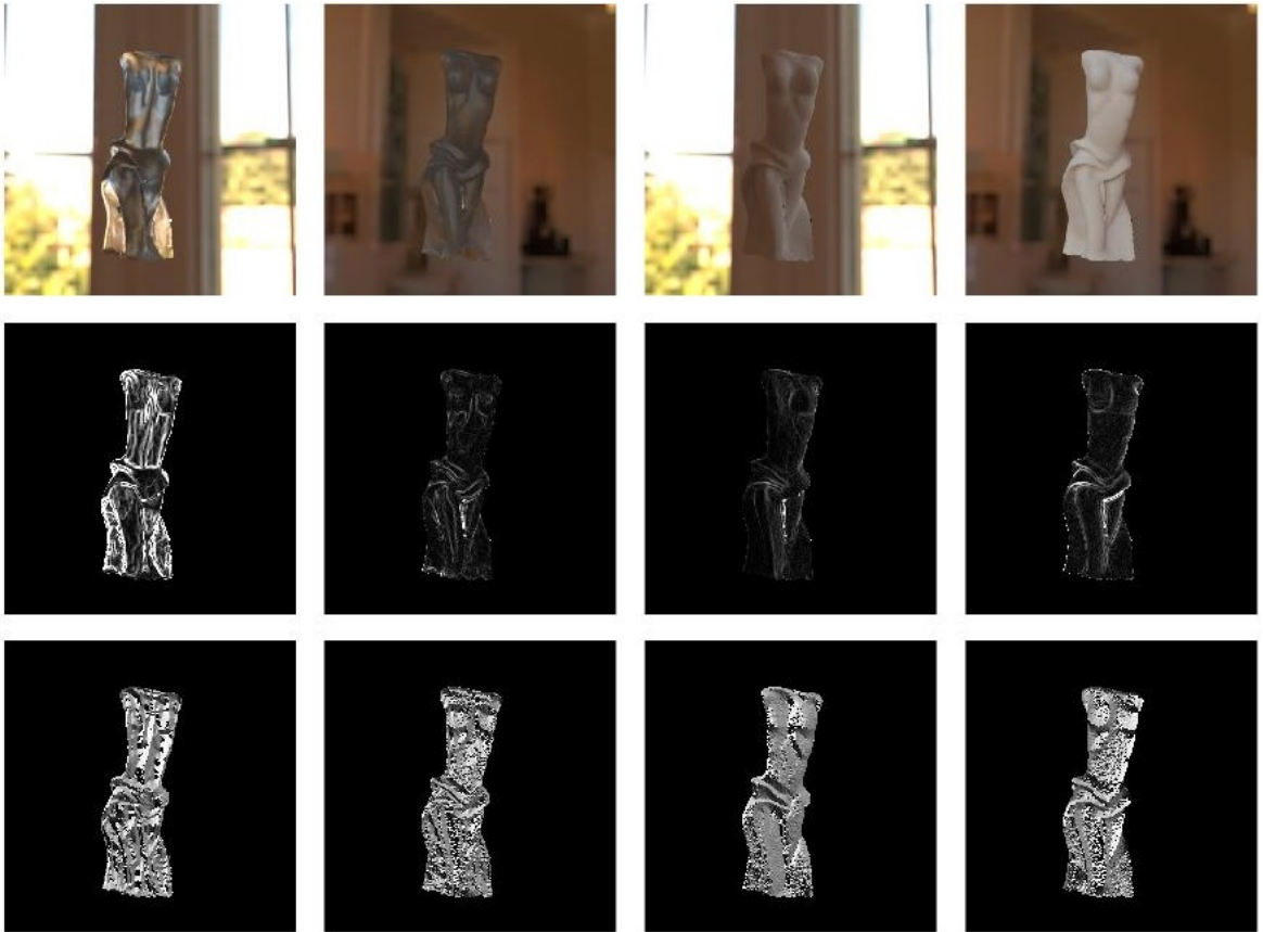
Figure 30: The top row illustrates the original images, the middle row shows the magnitude of the luminance gradient (the background is ignored), while the shades in the bottom row correspond to the gradient orientation. The back-lit translucent object has a high magnitude gradient, while it looks relatively homogeneous when front-lit. Under front light, a diffuse object produces more visible gradient (due to shading in the surface convexities) than a front-lit translucent one. In the front-lit condition, the gradient orientation closely follows the surface 3D geometry. When the objects are back-lit, the gradient orientation of an opaque object is strongly impacted by the partial side-illumination, while it looks more random for the back-lit translucent object, which also makes it difficult to recover its shape.
