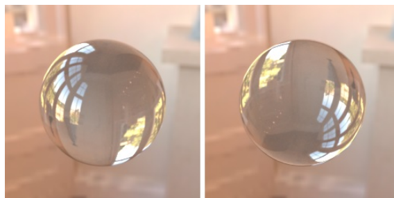
Figure 9: The transmission image in the left photograph is upside-down which indicates that it is the result of the refraction through a convex lens. If we simply rotate the sphere upside-down, then the transmission image will look more like an opaque mirror-reflection. This was first demonstrated by Kim & Marlow (2016) .
