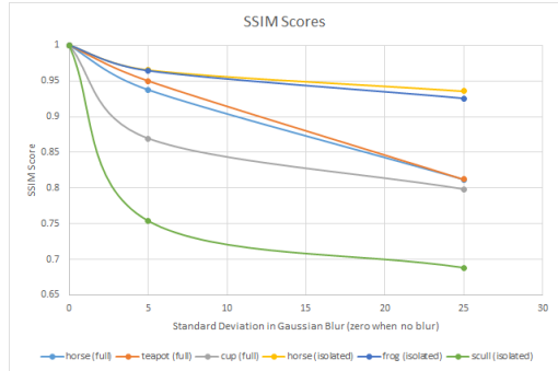
Figure 7. SSIM score as a function of the amount of blur
