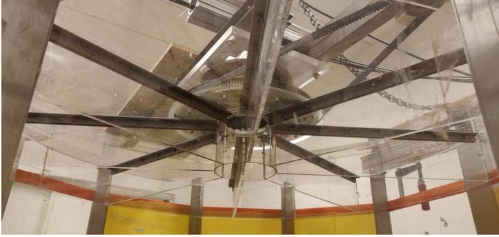
Figure 4.4: Image of the impeller used to rotate the water in the mixing tank.
