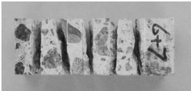
Figure 13: Subdivision of prism in 10 mm thick slices for determination of moisture profiles [35].
