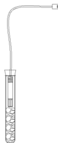
Figure 11: Measuring RH on a crushed concrete sample kept in a closed test tube [22].
